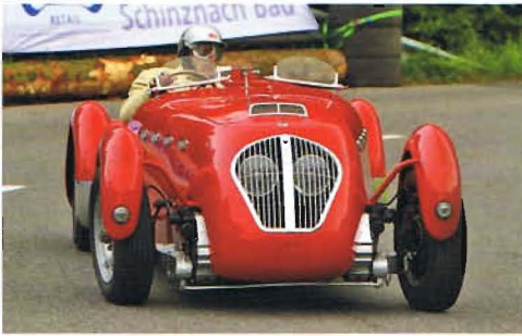
301 Healey Silverstone Type E Rennsportwagen 1950 Motor: Riley RMB 2443 ccm, 110 PS, 4 Zylinder
