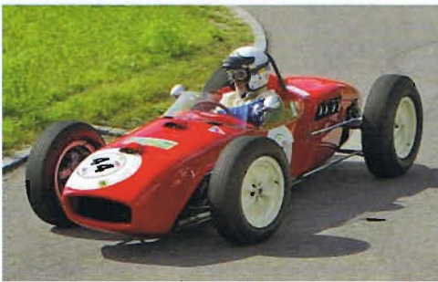
362 Lotus 18 Rennwagen Formel 1 1500 1960/61 Motor: Maserati 1500 1500 ccm, 150 PS, 4 Zylinder
