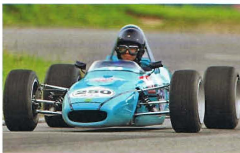
353 Merlyn Mk 10/14 Rennwagen Formel 3 1000 1967 Motor: Ford Novamotor (Basis Anglia) 1000 ccm, 110 PS, 4 Zylinder
