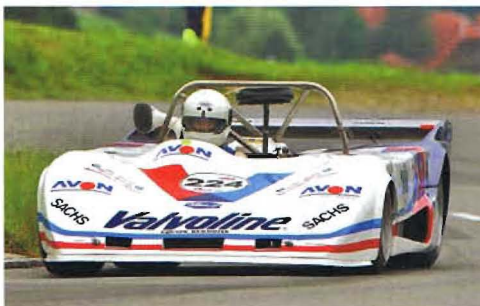
330 Lola T 297 Rennsportwagen 1978 Motor: BMW M 12 2000 ccm, 300 PS, 4 Zylinder Marcel Affentranger Lotzwil
