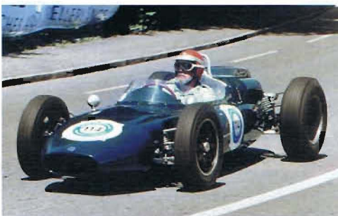
363 Cooper T 53 P Rennwagen Formel 1 1500 1961 Motor: Coventry Climax FPF 1500 1500 ccm, 145 PS, 4 Zylinder
